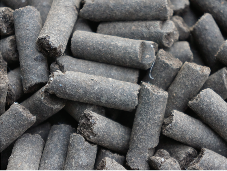
Fig. 6.7 Dried pellet from faecal sludge in Kampala, Uganda (photo credit: Moritz Gold)
