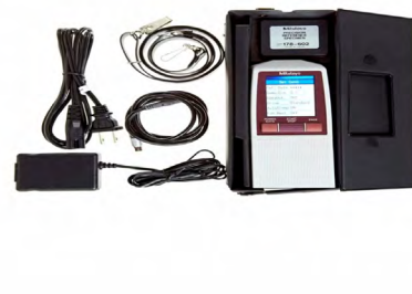
Figure 7: Surface profilometer for assessing surface roughness.
