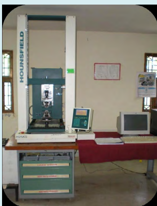
Figure 5: Universal testing machine for evaluation of Shear bond strength.
