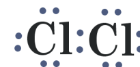
Figure 19.10: Two chlorine atoms share the pair of electrons between them to form a covalent bond.
