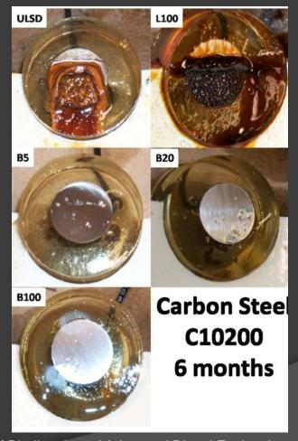
Source: Microbiological and Corrosivity Characterizations of Biodiesels and Advanced Diesel Fuels , Jason S. Lee, Richard I. Ray\*, Brenda J. Little, Naval Research Laboratory, 2009
