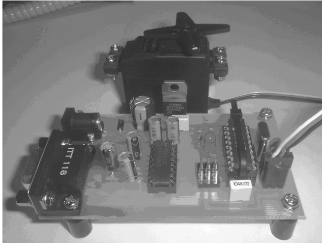
Figure 5. The PicServo controller (Roll 2000).
