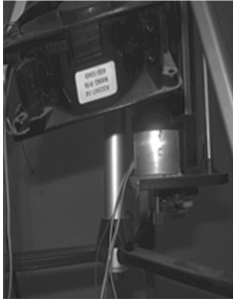
Figure 6. Stepper motor used for the Azimuth.
