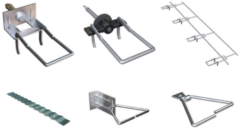
Fig. 1-19 Masonry veneer tie types. Top row, left to right: standard double eye and pintle plate tie, thermally optimized double eye and pintle screw tie, ladder eye-wire tie. Bottom row, left to right: corrugated masonry ties, adjustable L-bracket, nonadjustable surface-mounted tie.
