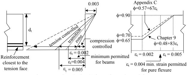
Fig. 1-2 Capacity reduction (\$\$) factors for Grade 60 reinforcement
