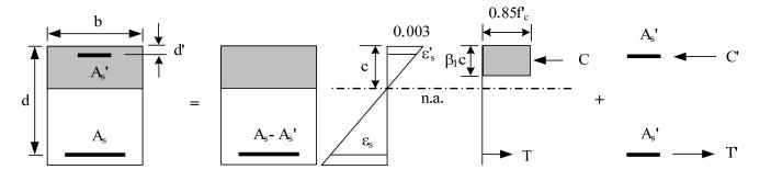
Fig. 1-3 A rectangular section with compression reinforcement
