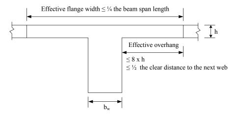
T-sections resulting from monolotically built slabs and beams
