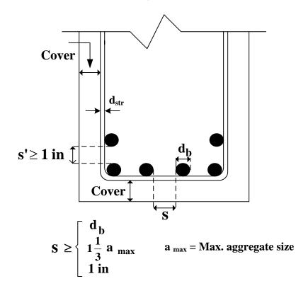
Flexure - 9 Bar spacing and cover requirements
