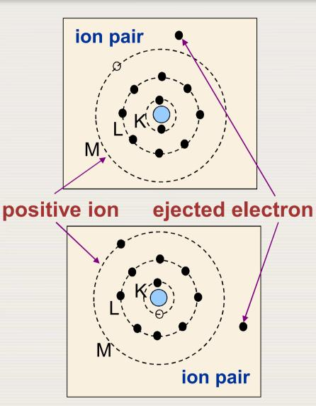
If the transferred energy exceeds the binding energy of the electron, ionization occurs, resulting in the electron ejected from the atom. An ion pair consisting of the ejected electron and the ionized, positively charged atom is then formed
