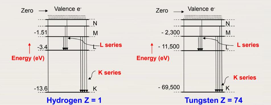
Energy levels for hydrogen and tungsten. Possible transitions between the various energy levels are shown with arrows
