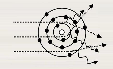
Bremsstrahlung photons are the major component of the X ray spectrum emitted by X ray tubes
