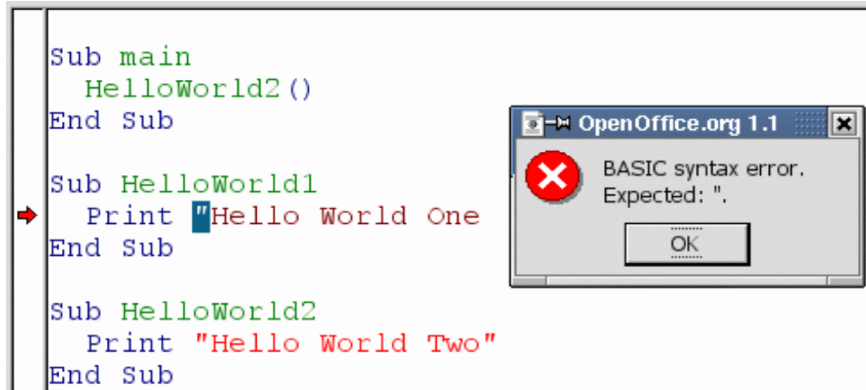
Figure 10. Click the Compile icon to find syntax errors such as a missing double quotation mark.
