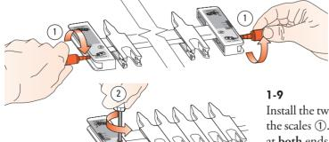
Install the two thumbscrews a few turns into the scales ①. Loosen the scale lock screw ② at **both** ends (by one turn only).
