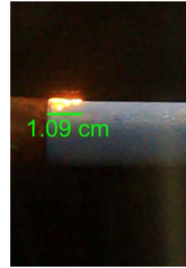
c) Arc is continuously compressed with 17 mph (7.65 m/s) wind injection
