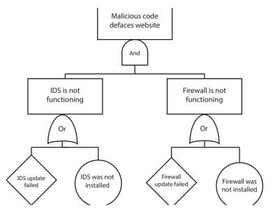
Figure 1-23: Fault tree for the cyber scenario.
