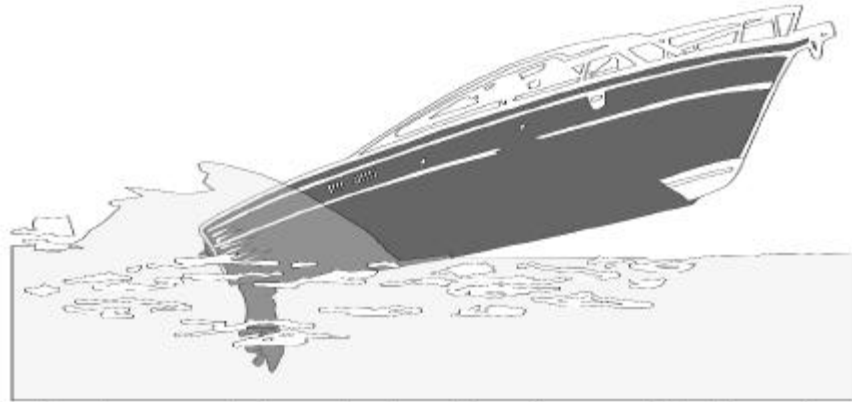
Excessive power applied causes stern to squat. Large stern wave and raised bow result. Coxswain loses forward visibility until craft attains planing mode.
