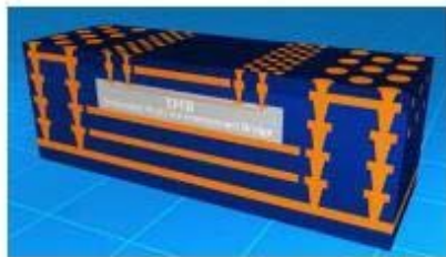
3) EMIB interconnect and HDI substrate FLI formation
