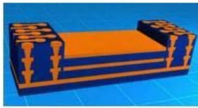
1) HDI substrate build-up to cavity layer
