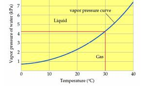
103. **Picture the Problem:** The liquid vapor curve shows the relationship between the vapor pressure and boiling point temperature of water.
