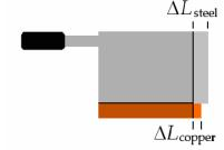
**Solution: 1.** Write the thermal expansion equations for copper and steel:
