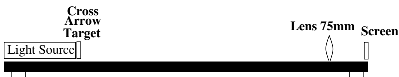
Figure 10.5: Arrangement of components for the approximate focal length measurement for a single lens.
