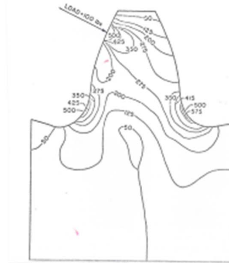
(b) Contour plot of isoclinic stress distribution in a gear tooth
