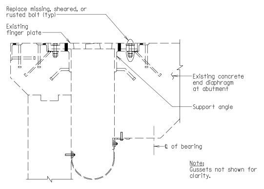
TYPICAL SECTION BETWEEN STRINGERS (ABUTMENT-SPAN SHOWN; SPAN-SPAN SIMILAR)
