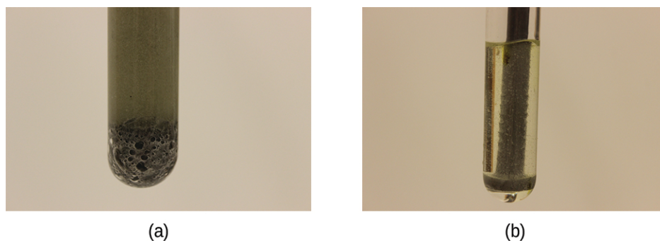
Figure 12.6 (a) Iron powder reacts rapidly with dilute hydrochloric acid and produces bubbles of hydrogen gas because the powder has a large total surface area: 2\text{Fe}(s) + 6\text{HCl}(aq) \longrightarrow 2\text{FeCl}_3(aq) + 3\text{H}_2(g) . (b) An iron nail reacts more slowly.
