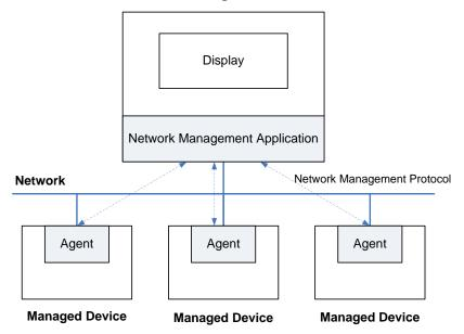
Figure 12.1: Typical Network Management Architecture [1]
