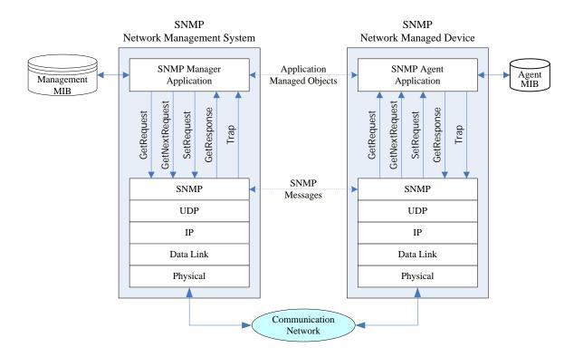
Figure 12.3: SNMP Network Management Architecture
