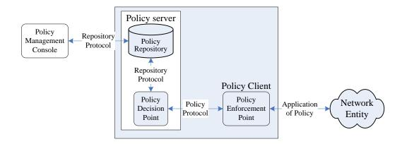
Figure 12.13: A Logic Architecture for PBNM
