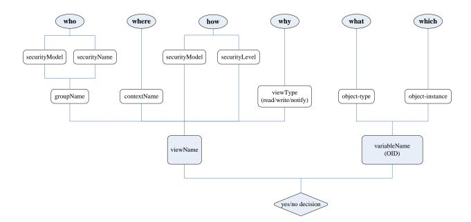
Figure 12.9: VACM Access Control Logic
