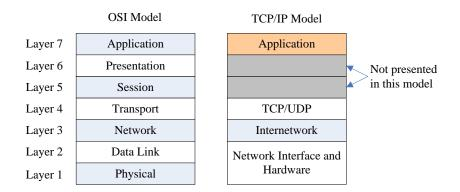
Figure 12.2: The OSI and TCP/IP Reference Models
