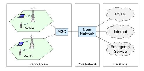
Figure 12.10: A Typical Cellular Network
