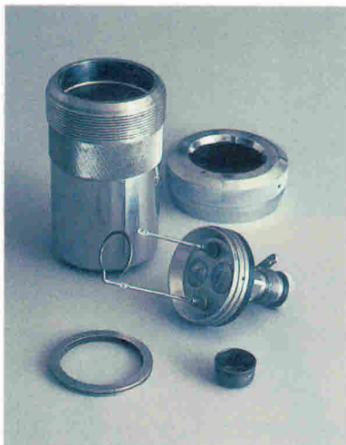
FIGURE 12–11. A calorimeter provides a closed, isolated system in which to measure energy transfer.
