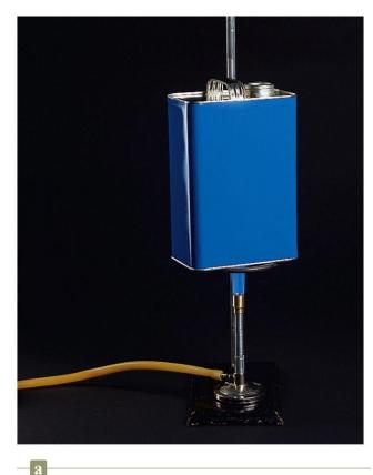
The pressure exerted by the gases in the atmosphere can be demonstrated by boiling water in a can and then turning off the heat and sealing the can.
