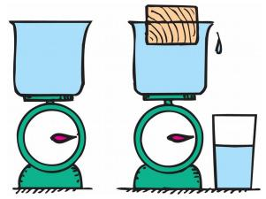
object floats, but some water spills out. How does the weight of the object compare with the weight of the water displaced?
