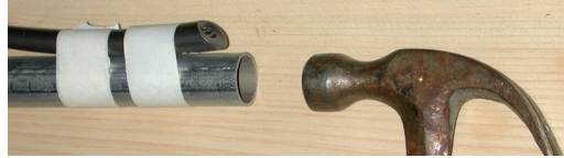
Figure 10 Microphone taped to steel pipe.
