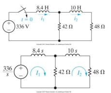
The voltage drop across the  $42\Omega$  resistor:
