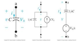
Configuration #2: an admittance sC in series with an independent voltage source  $V_0/s$
