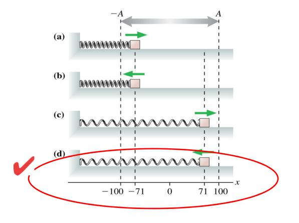
Four springs have been compressed from their equilibrium position at x = 0 cm. When released, they will start to oscillate. Rank in order, from highest to lowest, the maximum speeds of the oscillations.
