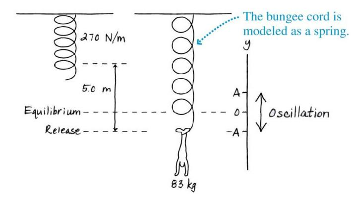
**SOLVE** Although the cord is stretched by 5.0 m when the student is released, this is *not* the amplitude of the oscillation. Oscillations occur around the equilibrium position, so we have to begin by finding the equilibrium point where the student hangs motionless. The cord stretch at equilibrium is given by Equation 14.41:
