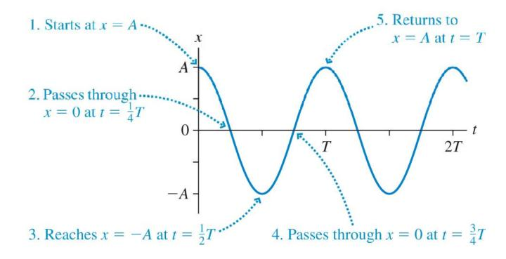
The oscillation frequency f is measured in cycles per second, or Hertz.
