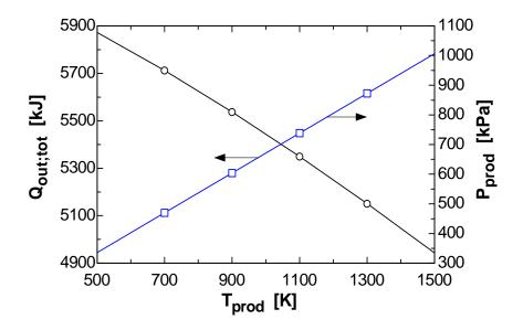
**15-71** Propane is burned with 50% excess air. The heat transfer per kmol of fuel is to be determined for given reactants and products temperatures.
