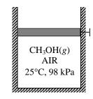
$$\overline{h}_{CO_2} + 2\overline{h}_{H_2O} + 5.64\overline{h}_{N_2} - 71.833 \times T_P = (1)(152,908) + (2)(127,952) + (5.64)(95,859) - (71.833)(2850) = 744,733 \text{ kJ} \text{ (Higher than 734,388 kJ)}$$
