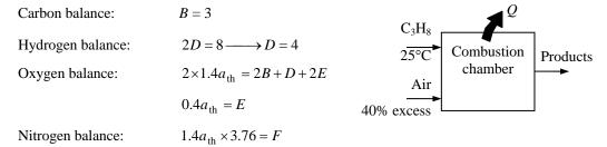
Solving the above equations, we find the coefficients (E = 2, F = 26.32, and  $a_{th} = 5$ ) and write the balanced reaction equation as
