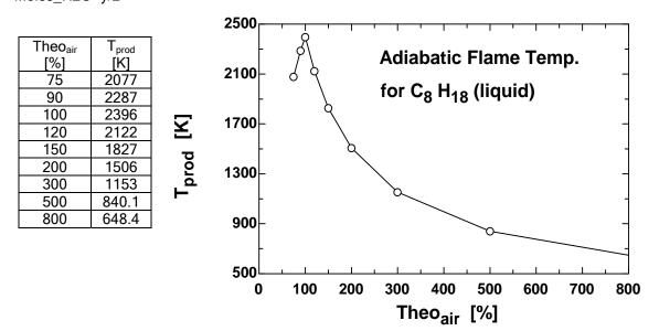
**15-128 EES** A general program is to be written to determine the adiabatic flame temperature during the complete combustion of a hydrocarbon fuel  $C_nH_m$  at 25°C in a steady-flow combustion chamber when the percent of excess air and its temperature are specified.
