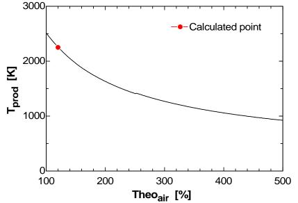
**15-81E** Hydrogen is burned with 20 percent excess air during a steady-flow combustion process. The exit temperature of product gases is to be determined.
