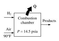
**15-102** A gaseous fuel with a known composition is burned with dry air, and the volumetric analysis of products gases is determined. The AF ratio, the percent theoretical air used, and the volume flow rate of air are to be determined.
