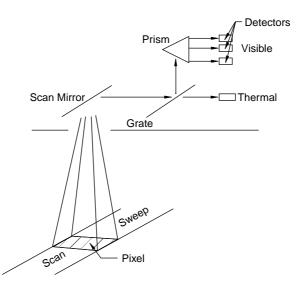
Figure 15.4 Rudimentary components of an MSS.
