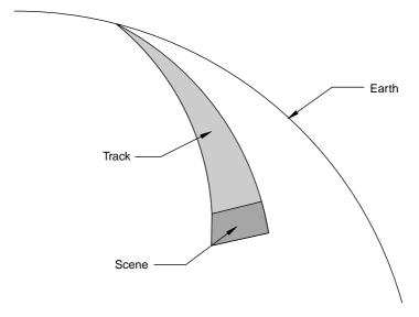
Figure 15.2 A scene from a scanner's orbital path.
