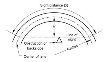
Where: S = Sight distance (ft) R = Centerline radius of inside lane (ft) M = Distance from inside lane centerline (ft)
