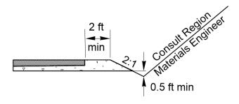
Example 3: Cut section with ditch
