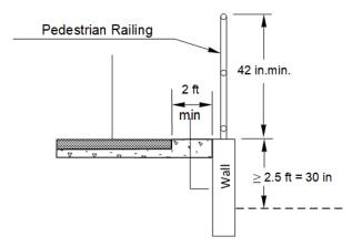
Example 4: Railing used at drop off
