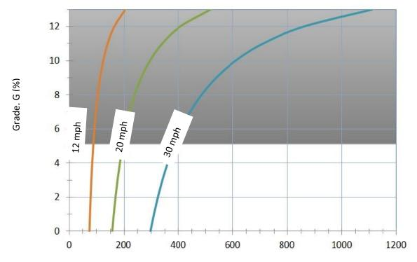
Stopping Sight Distance, S (ft) (Based on 2.5 second reaction time)
