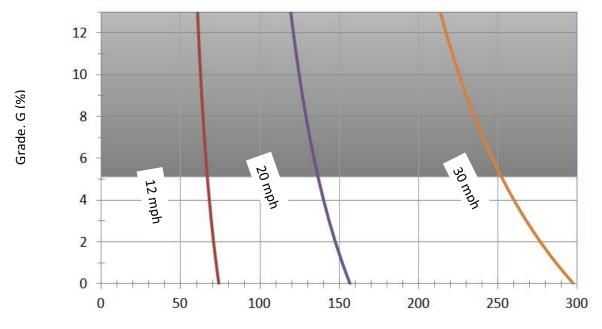
Stopping Sight Distance, S (ft) (Based on 2.5 second reaction time)
