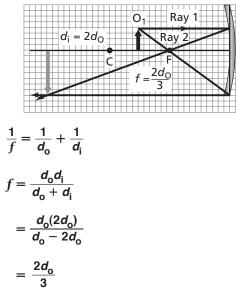
Draw and label a ray diagram showing the location of the object if the image is located twice as far from the mirror as the focal point. Prove your answer mathematically. Calculate the image height as a function of the object height for this placement.
