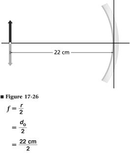
**89. Use Equations** Show that as the radius of curvature of a concave mirror increases to infinity, the mirror equation reduces to the relationship between the object position and the image position for a plane mirror.
