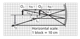
**83.** A ball is positioned 22 cm in front of a spherical mirror and forms a virtual image. If the spherical mirror is replaced with a plane mirror, the image appears 12 cm closer to the mirror. What kind of spherical mirror was used?
