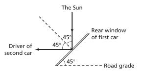
The Sun's position directly overhead would likely reflect light into the driver's eyes, according to the law of reflection.
