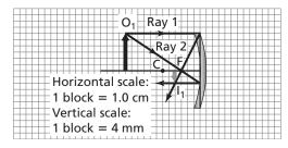
**b.** Use the mirror equation to calculate the image position.
