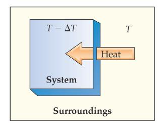
In a reversible process the system changes in such a way that the system and surroundings can be put back in their original states by exactly reversing the process.
