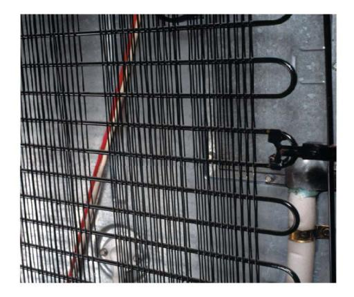
These cooling coils are the refrigerator's high-temperature heat exchanger. Heat energy is being transferred from hot gas inside the coils to the cooler room air.
