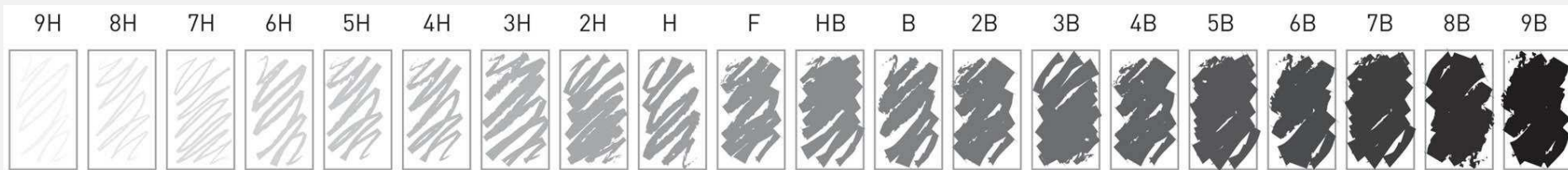
2.4 Pencil hardness scale from 9H to 9B
