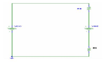
• REI in the above circuit is  $(\beta+1)RE$  which means that, the emitter resistance that is common to both the loops appears as such a high resistance in the input loop.
