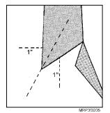
Figure 2-5. Proper positioning of collar devices.
