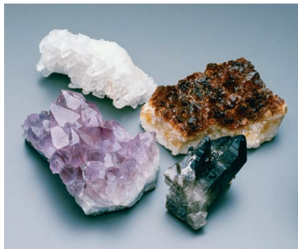
◆ Figure 2.12 Because of the presence of slight impurities, minerals, such as quartz, can occur in a wide range of colours. (Photo courtesy of E. J. Tarbuck)
