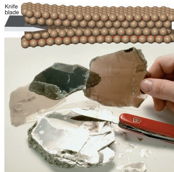
◆ Figure 2.14 The thin sheets shown here were produced by splitting a mica (muscovite) crystal parallel to its perfect cleavage. (Photo by Chip Clark)
