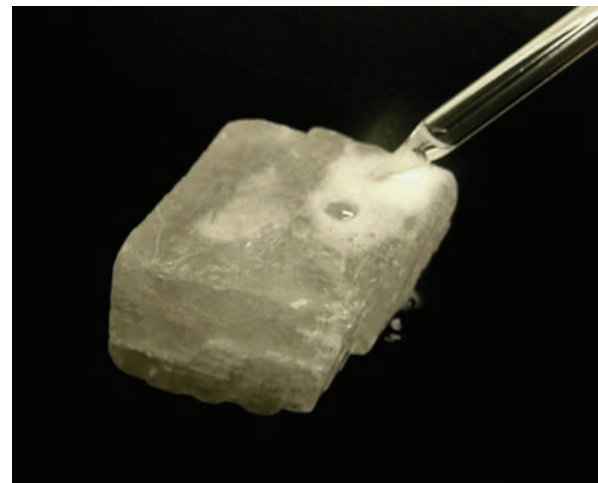
◆ Figure 2.19 Calcite vigorously effervesces when brought into direct contact with acid. (Photo by C. Tsujita)
