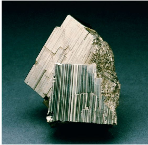
◆ Figure 2.11 Crystal form is the external expression of a mineral's orderly internal structure. A. Pyrite, commonly known as "fool's gold," often forms cubic crystals. They may exhibit parallel lines (striations) on the faces. B. Quartz sample that exhibits well-developed hexagonal crystals with pyramid-shaped ends. (Photo A courtesy of E. J. Tarbuck; photo B by Breck P. Kent)
