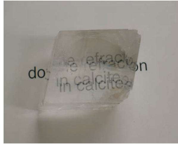
◆ Figure 2.18 A transparent specimen of calcite showing the property of double refraction. (Photo by S. R. Hicock)
