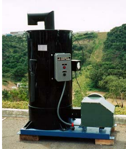
Figure 2.26 Photo of an Activated Carbon Odor Control System
