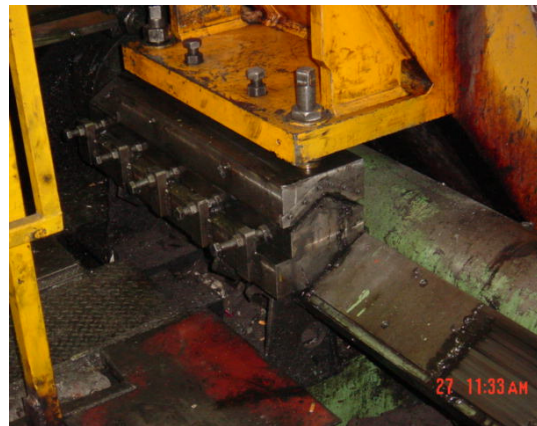
Figure 2-17: Container guides modified to V-type
