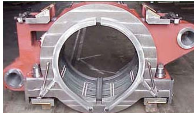
Figure 2-14: Conversion of container guides to flat type (Photo courtesy of Lake Park Tool)
