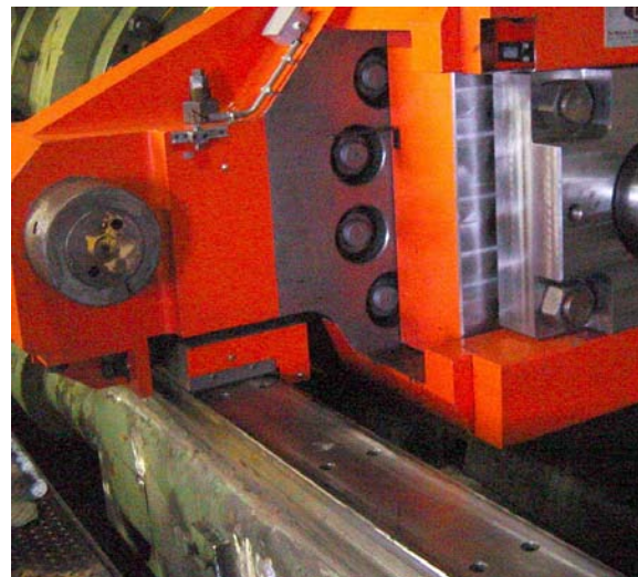
Figure 2-15: Conversion of X container guides to horizontal (Photo courtesy of OMAV)
