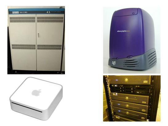
Figure 2.3: Different systems and architectures running Unix. A VAX-11 by DEC (VAX), an O2 by SGI (MIPS), a Mac Mini by Apple (PowerPC), PowerEdge servers by Dell (x86).
