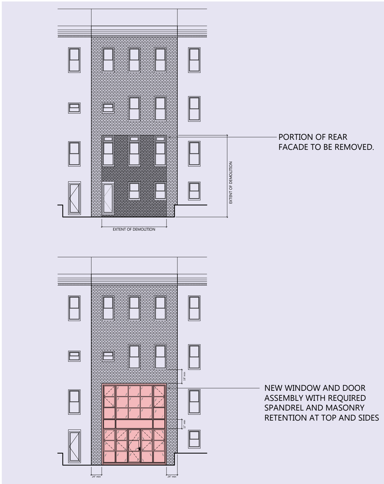
A sample drawing for combining window openings horizontally and vertically at the bottom two floors of a non-visible secondary facade.
