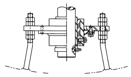
**Figure 21-33** Tripod steady bearing detail. (Courtesy of Chemineer.)
