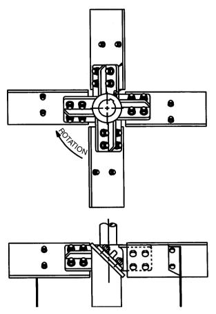
**Figure 21-37** Pitched blade turbine with bolted blades and stabilizers. (Courtesy of Chemineer.)
