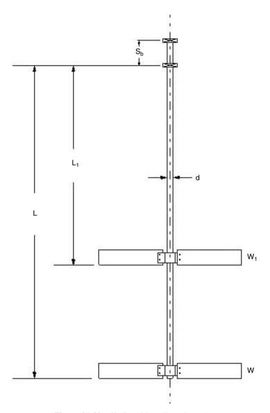
Figure 21-32 Shaft and impeller schematic.
