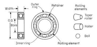
Figure 21-19 Bearing components.
