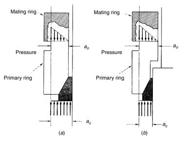
**Figure 21-29** (a) Unbalanced and (b) balanced mechanical seals.
