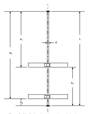
Figure 21-34 Shaft and impellers with steady bearing.
