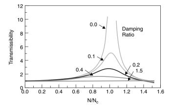
Figure 21-36 Transmissibility for various damping ratios.
