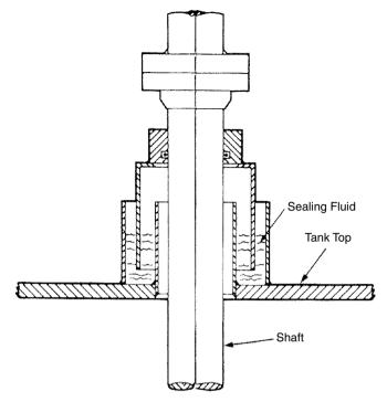
Figure 21-31 Hydraulic seal. (Courtesy of Lightnin.)
