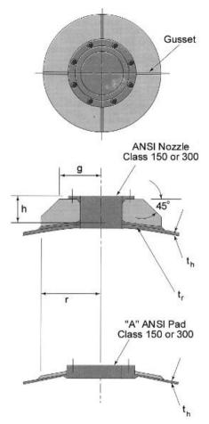
**Figure 21-44** Reinforcement for nozzles and pads. (Fasano et al., *Chemical Engineering Progress*, 1995 © AIChE.)
