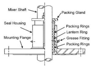
Figure 21-26 Stuffing box shaft seal. (Courtesy of Chemineer.)
