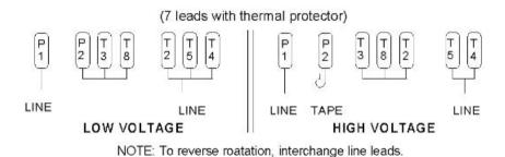
Figure 21-12 Typical wiring for single-phase motors. (Courtesy of Chemineer.)
