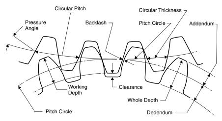
Figure 21-15 Basic gear mesh. (Courtesy of Hamilton Gear.)
