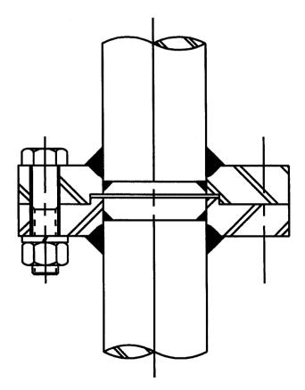
Figure 21-40 Welded shaft coupling. (Courtesy of Chemineer.)
