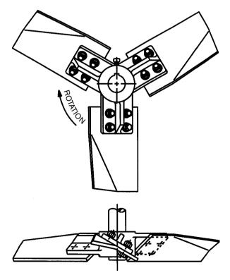
Figure 21-38 Hydrofoil impeller with bolted blades. (Courtesy of Chemineer.)
