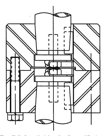
Figure 21-41 Removable shaft coupling. (Courtesy of Chemineer.)
