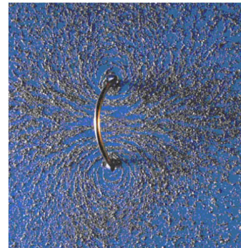
Magnetic field lines in the vicinity of a circular coil carrying a current.
