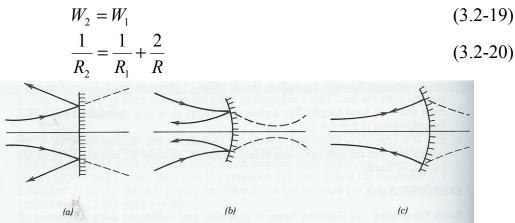
**Figure 3.2-8** Reflection of a Gaussian beam of curvature  $R_1$  from a mirror of curvature R: (a)  $R = \infty$ ; (b)  $R_1 = \infty$ ; (c)  $R_1 = -R$ . The dashed curves show the effects of replacing the mirror by a lens of focal length f = -R/2.
