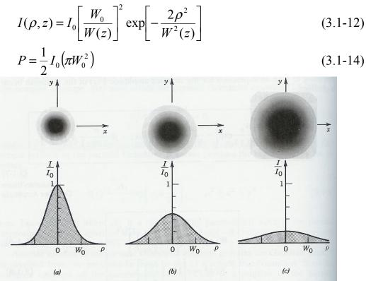
**Figure 3.1-1** The normalized beam intensity  $I/I_0$  as a function of the radial distance  $\rho$  at different axial distances: (a) z = 0; (b)  $z = z_0$ ; (c)  $z = 2z_0$ .
