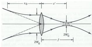
Figure 3.2-3 Focusing a beam with a lens at the beam waist.
