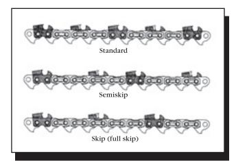
Figure 3-6—The cutter sequences for three types of chains: standard, semiskip, and skip (full skip).—Oregon Maintenance and Safety Manual, permission by Blount, Inc.
