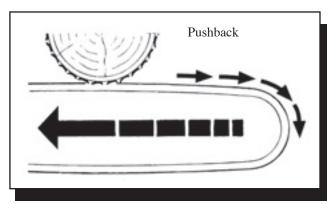
Figure 3-19—Pushback occurs when the chain on the top of the bar is suddenly stopped by contacting another object or by being pinched.—From Chain Safety Manual, permission by Stibl, Inc.
