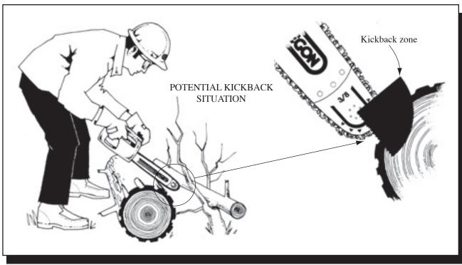
Figure 3-18—Kickback occurs when the upper quadrant of the bar nose contacts a solid object or is pinched.—Oregon Maintenance and Safety Manual, permission by Blount, Inc.
