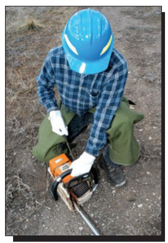
Figure 3-17—Start the saw on firm ground.
