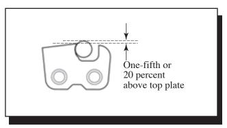
Figure 3–11—Hold the file at least one-fifth of the file's diameter above the cutter's top plate.—Oregon Maintenance and Safety Manual, *permission by Blount, Inc.*
