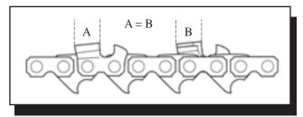
Figure 3-14—All cutters should be the same length.—Oregon Maintenance and Safety Manual, *permission by Blount, Inc.*
