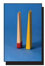
Figure 3-22—Double-taper wedges are designed to reduce bind.
