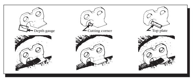
Figure 3-9—The depth gauge controls the depth at which a tooth's cutting corner bites into the wood.—Oregon Maintenance and Safety Manual, permission by Blount, Inc.
