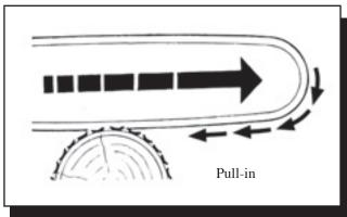
Figure 3-20—Pull-in occurs when the chain on the bottom of the bar is suddenly stopped by contacting another object or by being pinched.—From Chain Safety Manual, permission by Stibl, Inc.
