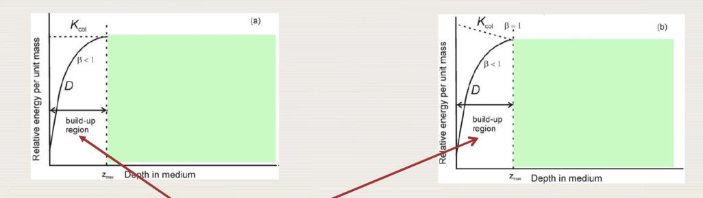
There is a build-up region for the dose, at small depths in the medium. The build-up region has dimensions  $(z_{max})$  similar to the range of the charged particles in the medium
