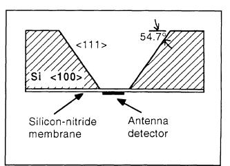
**Figure 1.** Example of anisotropic etching in a <100> silicon wafer. The opening of the wafer yields a pyramidal horn with a flare angle of  $35.5^{\circ}$ .
