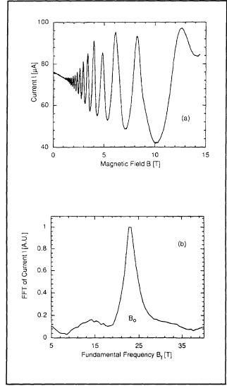
**Figure 11.** (a) Tunneling current (at a fixed bias voltage) as a function of the strength of a magnetic field applied in the same direction as that of the tunneling current. (b) Fourier transform of the tunneling current as a function of 1/B.
