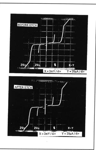
Figure 4. DC I-V curves for a device on SiN membrane (top) before etching, and (bottom) after etching the Si wafer in KOH.
