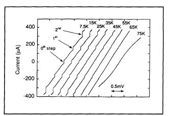
Figure 8. I-V curves of the high- $T_c$  Josephson junction irradiated by coherent radiation at 176 GHz and taken at different temperatures. Shapiro steps are still visible at 65 K.
