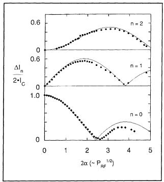
**Figure 9.** Measured amplitudes (normalized by the critical current in the absence radiation) of the zeroth, first, and second Shapiro steps as functions of the square root of radiation power at 176 GHz near 5 K. The solid lines are Bessel functions.
