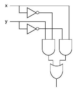
\*24. Construct the XOR operator using only NAND gates. Hint: x XOR y = ((x ' y)' (xy')')'
