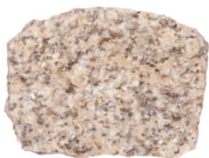
Figure 6 A Granite is an intrusive igneous rock that forms when magma cools slowly beneath Earth’s surface. B Rhyolite is an extrusive igneous rock that forms when lava cools quickly at Earth’s surface.
