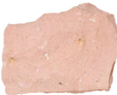
Figure 6 A Granite is an intrusive igneous rock that forms when magma cools slowly beneath Earth’s surface. B Rhyolite is an extrusive igneous rock that forms when lava cools quickly at Earth’s surface.
