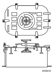
Figure 3-10. Raised watertight hatch with scuttle.
