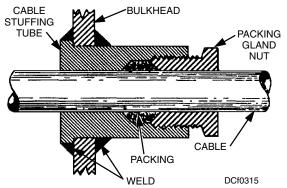
Figure 3-15. Cable penetration through watertight bulkhead.
