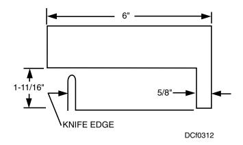
Figure 3-12. Gauge for measuring knife-edge height.
