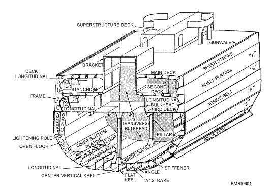
Figure 3-1. Illustrative hull structure.
