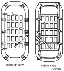
Figure 3-7. Quick-acting watertight door.
