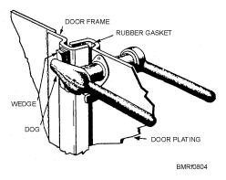
Figure 3-14. Watertight door parts.
