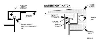
Figure 3-13. Gasket inspection.
