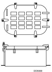
Figure 3-9. Raised watertight hatch.
