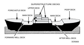
Figure 3-3. Weather decks.
