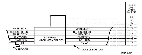
Figure 3-4. Deck numbering system.
