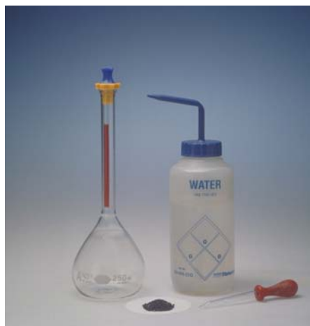
The materials required to make a solution by direct addition
