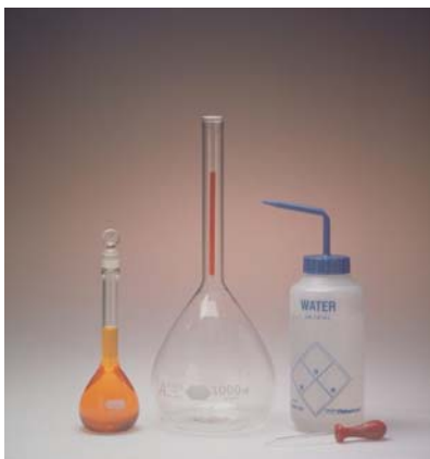
The materials required to make a solution by dilution
