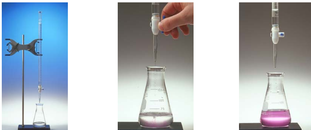
The titration of tartaric acid with sodium hydroxide
