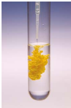
The precipitation of lead iodide
